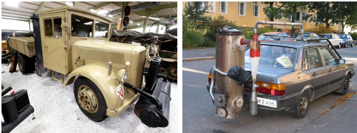
Picture 1: Wood fired gasifier to fuel trucks and cars; left: © AlfvandBeem, right: © Abc10
