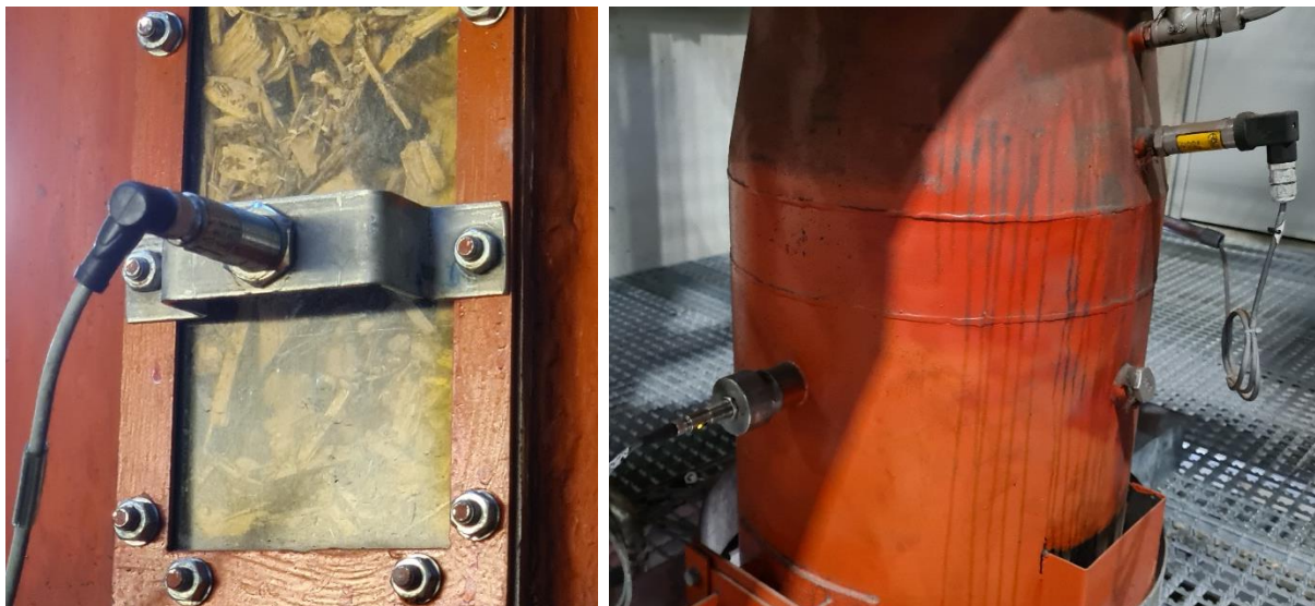
Picture 29: Sensor to check the filling level and to secure the feedstock conveying system
