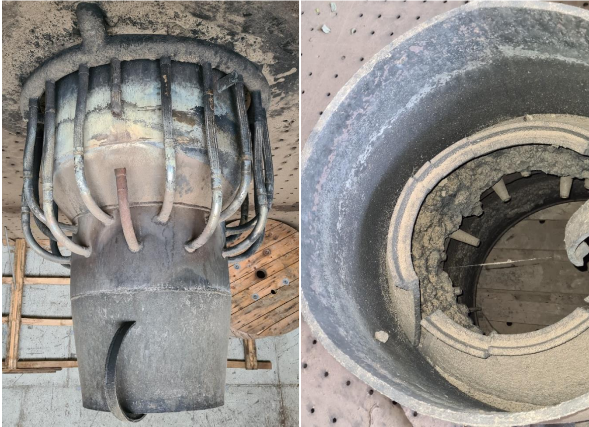
Picture 13: Downdraft fixed bed gasifier: left: coat of gasifier with air pipes; right: insight from bottom
