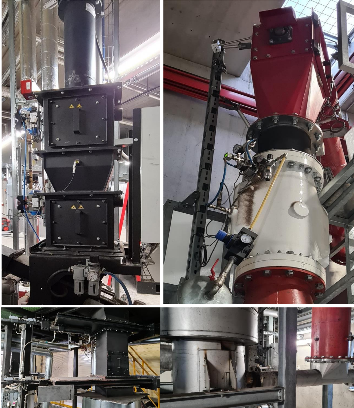
Picture 7: Safety devices upfront of the gasifier: top left: double valves; top right: combination of slider and air cushion; bottom left: double slider; bottom right auger screw into gasifier
