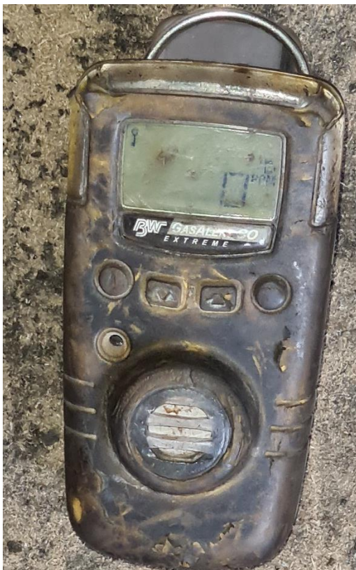
Picture 35: Handheld safety device to detect different types of gases (toxic, explosive)
