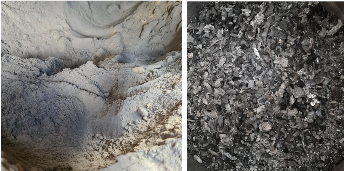
Picture 26: Left: ash of full combusted wood; right: raw charcoal
