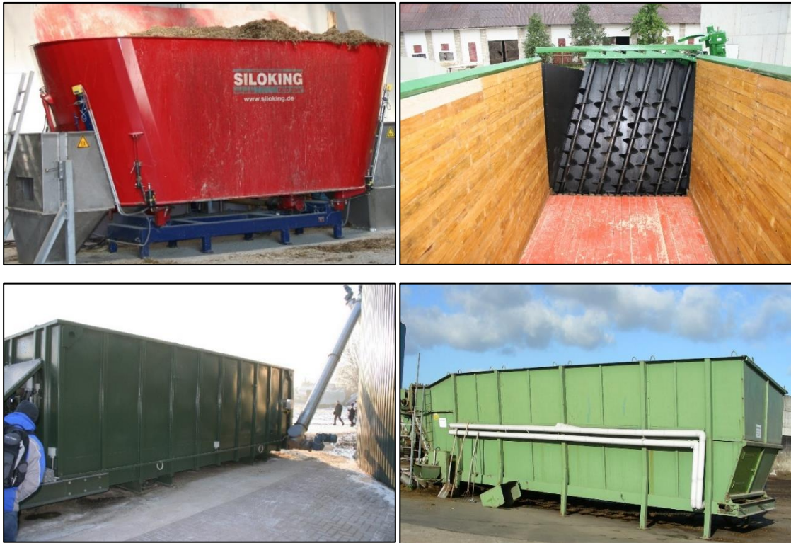
Picture 10: Substrate feeder systems for bulky and dry substrates: top left: with internal mixing screws, top right: feeding system with walking floor, bottom left: push floor, bottom right: scraper floor.
