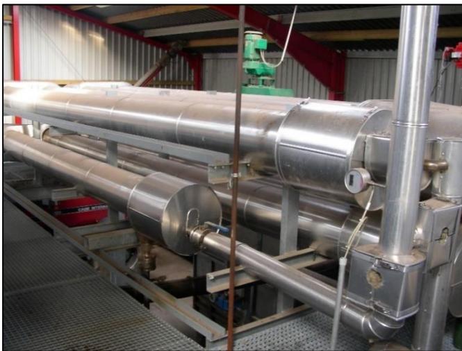
Picture 8: Steam explosion, left: continuously processed, right: batch system.
