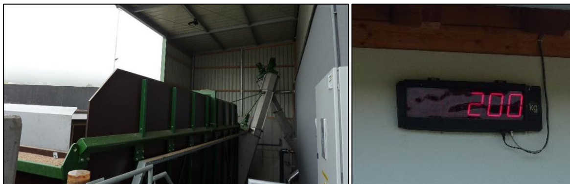
Picture 45: Feeder for bulky substrates with included weighing unit and big display also directly on the device so staff has control when loading the feeder.
