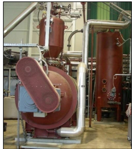
Picture 8: Steam explosion, left: continuously processed, right: batch system.
