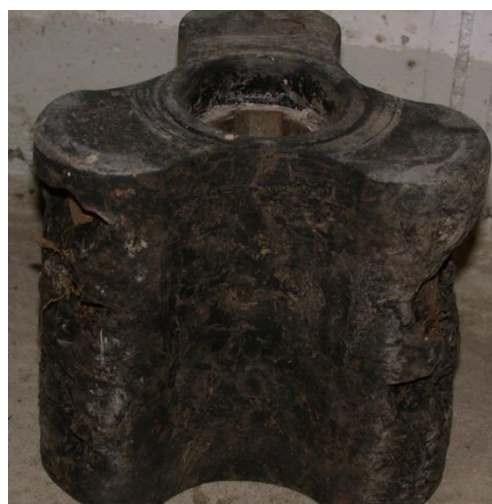
Picture 34: Left: piston of a rotary displacement pump, Right: Damaged piston through impurities like stones.
