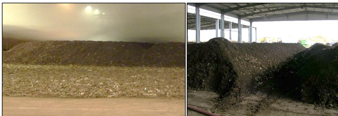
Picture 53: Post-composting of digestate from a dry fermentation process; left: in a closed hall with automatic aeration through the compost windrow and collection and cleaning of exhaust air in a biofilter, right: windrow post-composting in an open hall.
