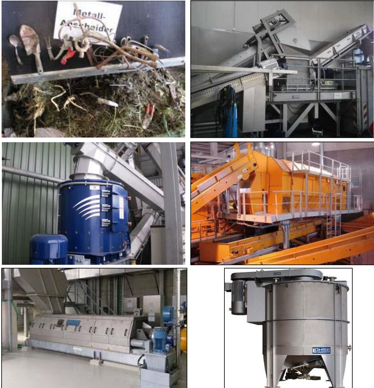
Picture 6: Metal separation is always the first step before further treatment, followed by crushing and further separation like sieving, separation through decanter or pulper.
