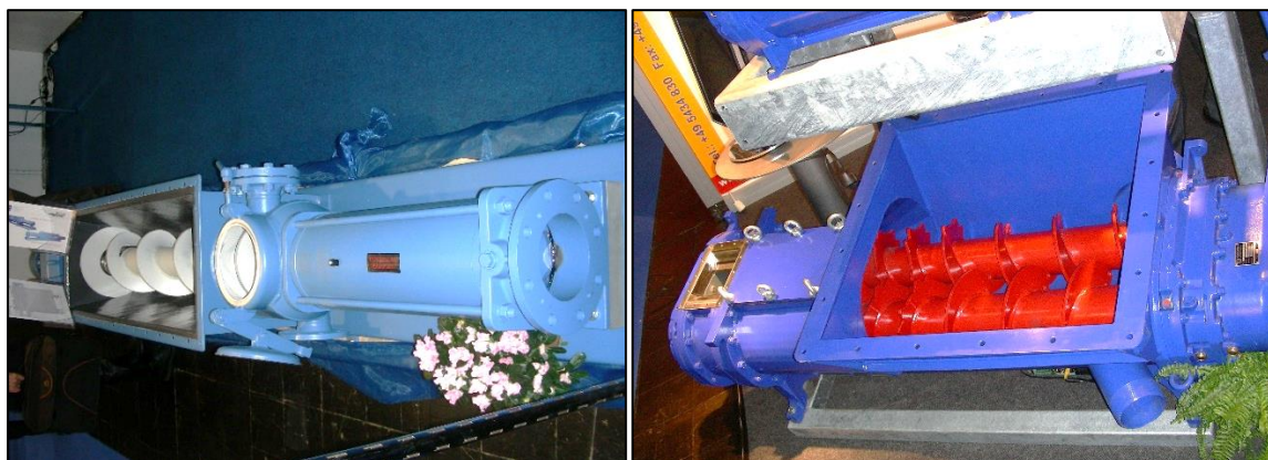
Picture 13: Pumps with a screw conveyor in front to mix solid and liquid substrate before pumping it into the digester, left: eccentric spiral pump, right: rotary piston pump.
