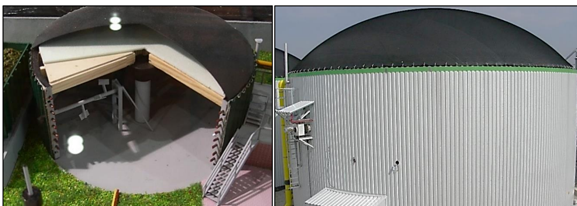
Picture 58: left: cross section of a model with single membrane; right: digester with single EPDM membrane.
