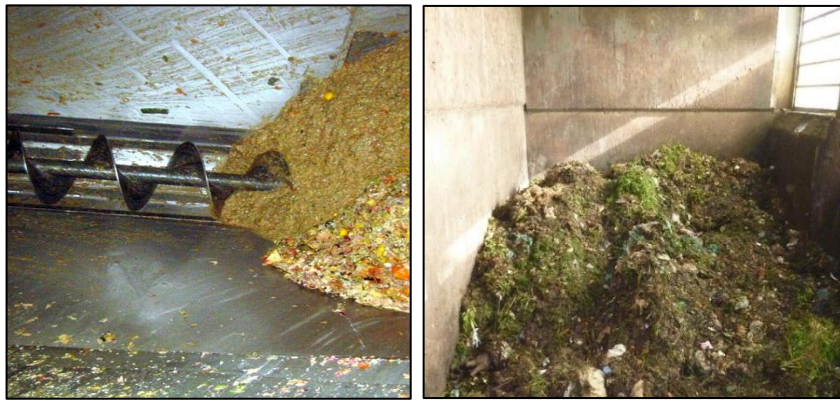
Picture 4: Bunker systems for solid organic waste with two different conveying systems, left: screw conveyor, right: crane.
