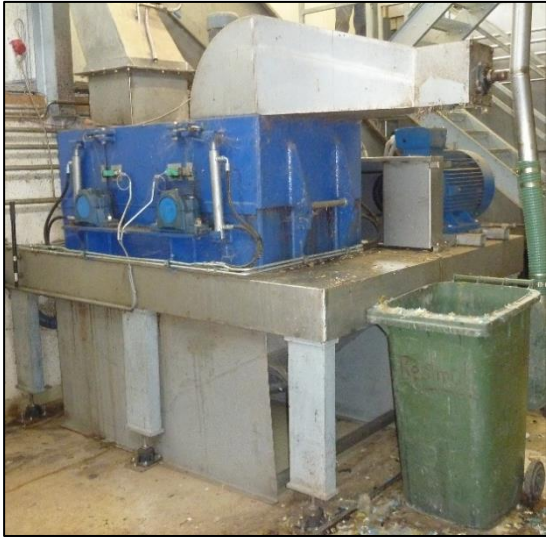
Picture 7: Left: unpacking machine for expired food with automatic separation of impurities, right: sanitation devices installed in parallel for higher performance.
