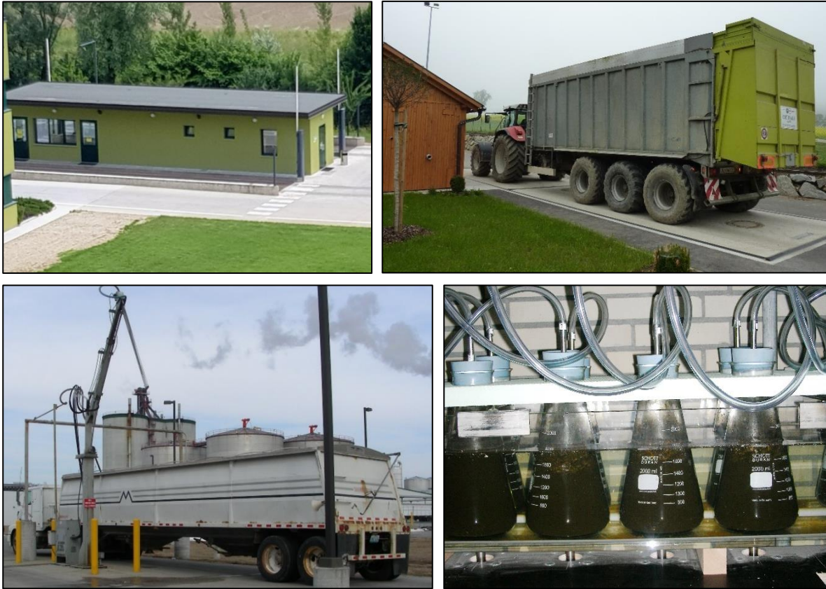
Picture 1: top: office to check delivered feedstock and weighbridge, bottom left: automatic sampling-taking of delivered feedstock, bottom right: batch test determining the methane yield of specific substrates.
